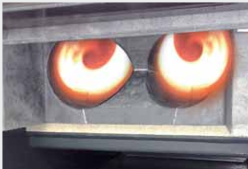
Highly efficient due to the double vortex combustion chamber
