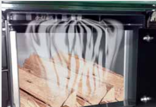
Smoke extraction via open filling shaft door
